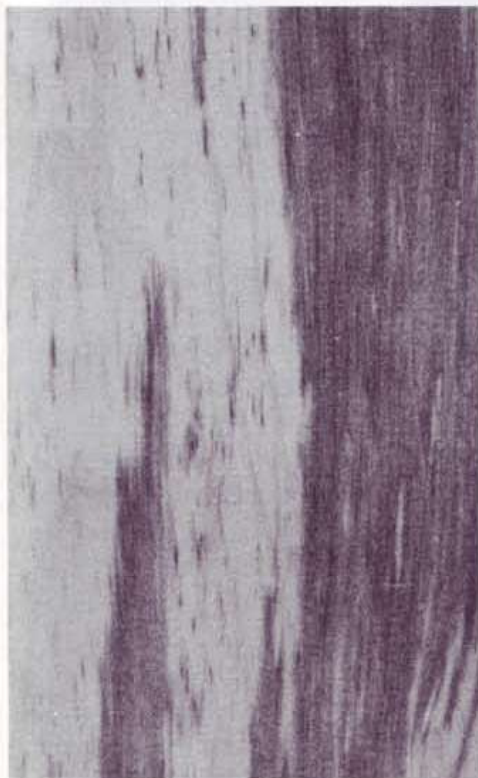
Blue stain: Gray-blue color caused by a fungus which attacks the sapwood before it is fully dry.
